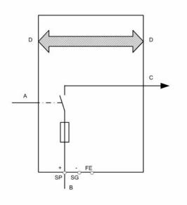
On the PI module the system power present (A) is interrupted and re-established (B). This creates a new power supply segment (C). To do this both A and B should be present therefore. The internal communication signals (D) are transferred as normal.
